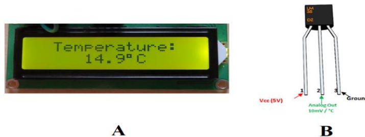
Fig. 3. Temperature sensor output with LCD display output
