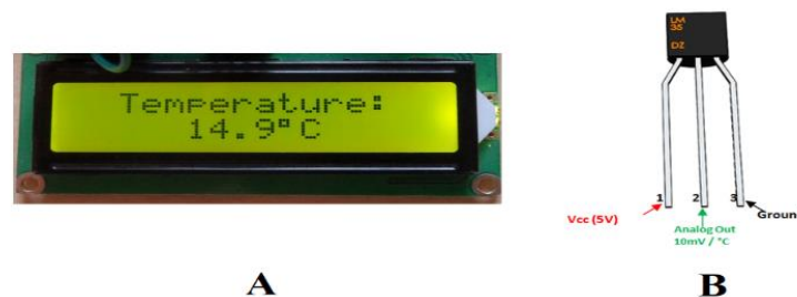
Fig. 3. Temperature sensor output with LCD display output
