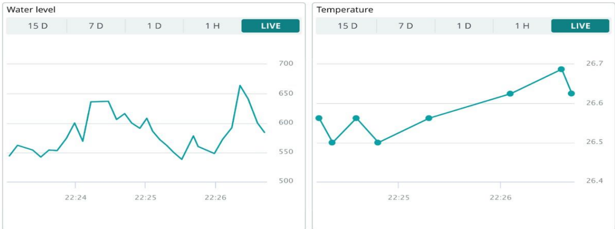
Fig .5. Live data of Water-Level Sensor & Temperature Sensor
