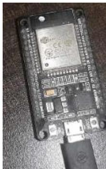
Fig. 8. ESP32 Controller
