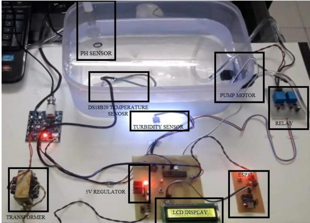
Fig. 9. Prototype model of the proposed model.
