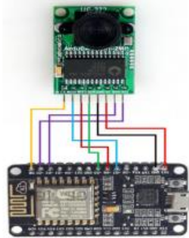
Fig. 5. ESP8266 with connected Camera
