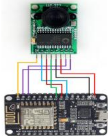
Fig. 5. ESP8266 with connected Camera
