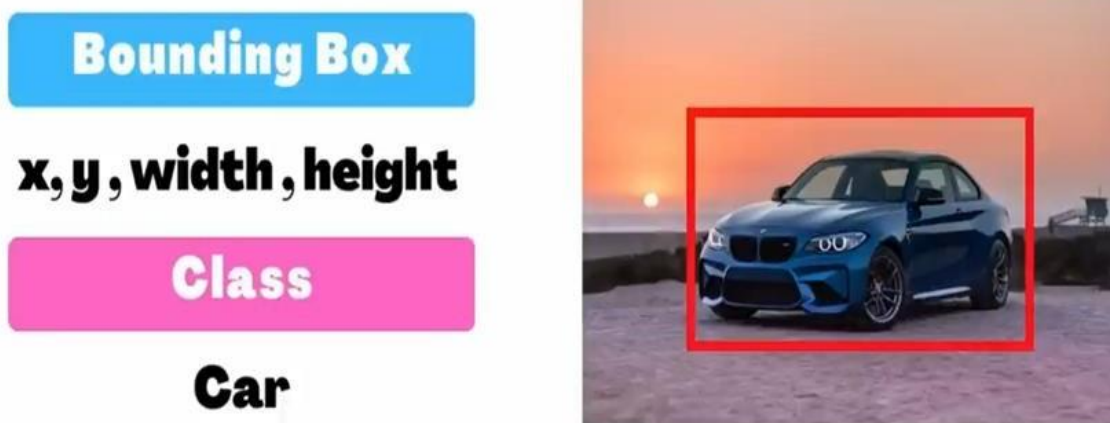
Fig. 2. The main two contents of the object detection process: bounding box and the class.
