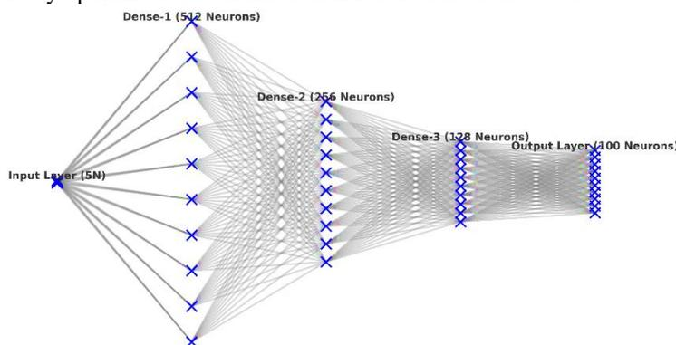
Fig. 3. FFNN Architecture for IoT-Driven Healthcare Data Transmission.
