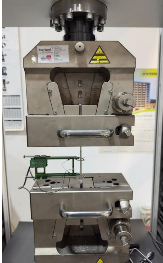
Fig. 3. Tensile testing arrangement for the produced AA6061-T6
