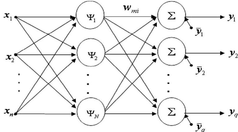
Fig.3. Structure of wavelet neural network
