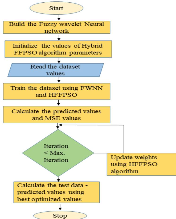
Fig .2. Flowchart of FWNN and HFFPSO algorithm
