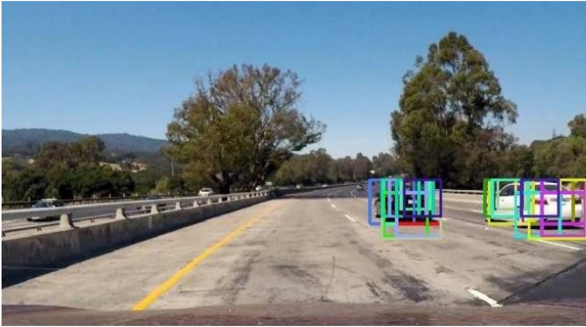
Fig. 8. Sliding window with the refined sliding windows
