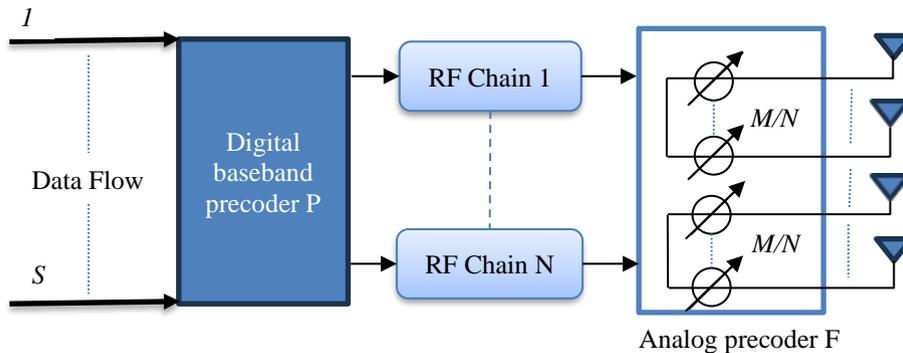
Fig. 3. Hybrid precoding system structure
