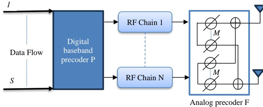
Fig. 2. Hybrid precoding system structure[35]
