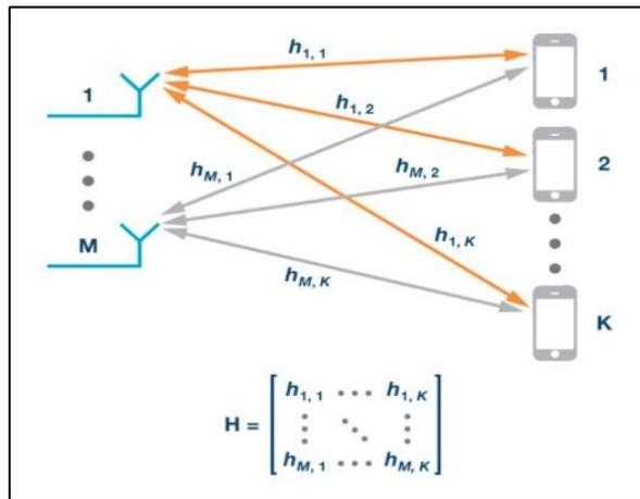
Fig. 1. Channel state information is required to characterize a massive MIMO system[16].
