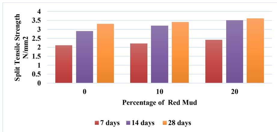
Fig.5. Split tensile strength on concrete
