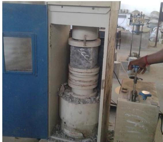
Fig.1. Compressive test on cube
