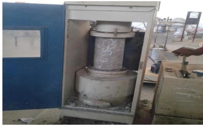
Fig.4. Compressive test on cube
