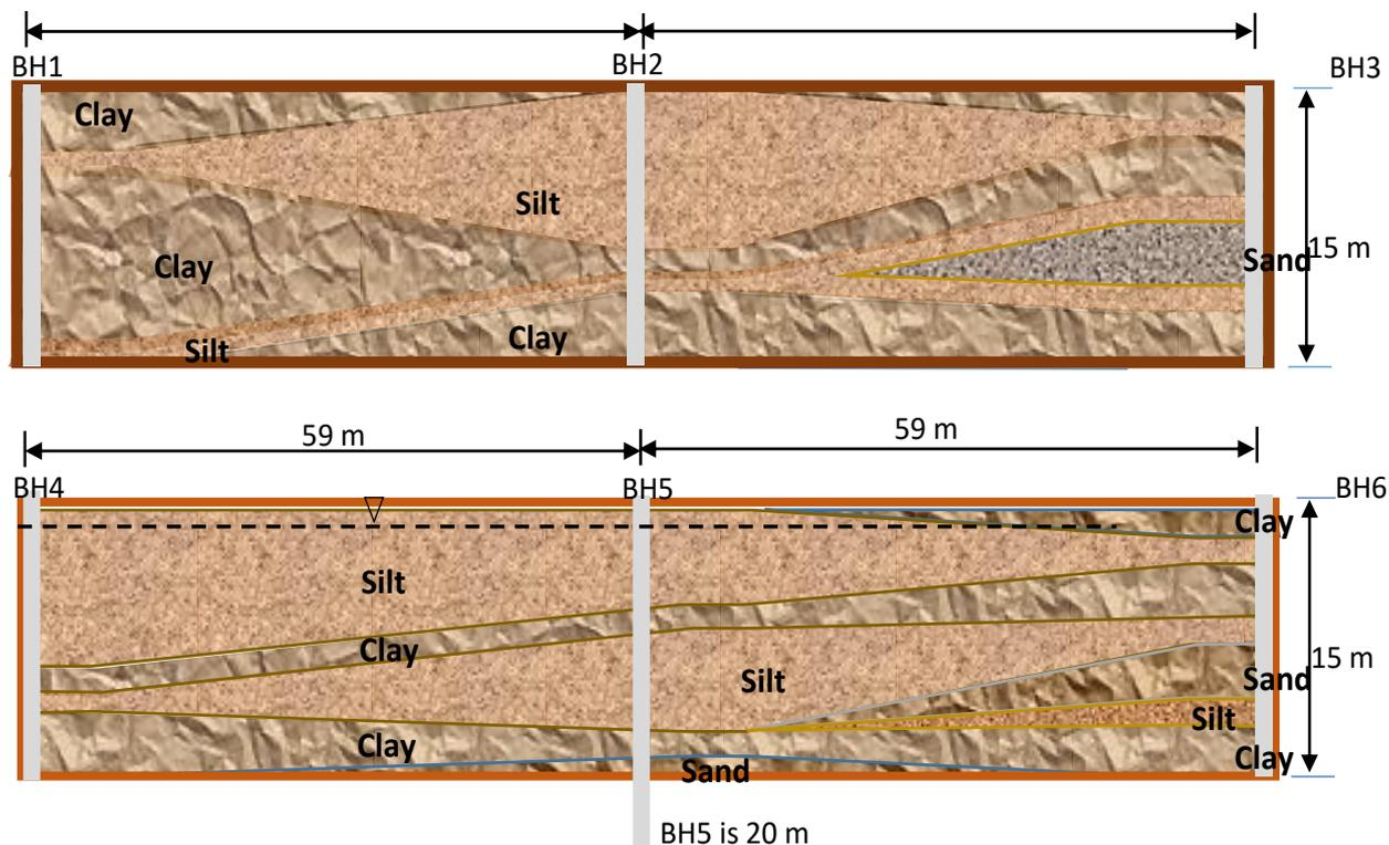
Fig. 3. (a,b): Soil Profile of Section through Boreholes 4, 5, and 6.
