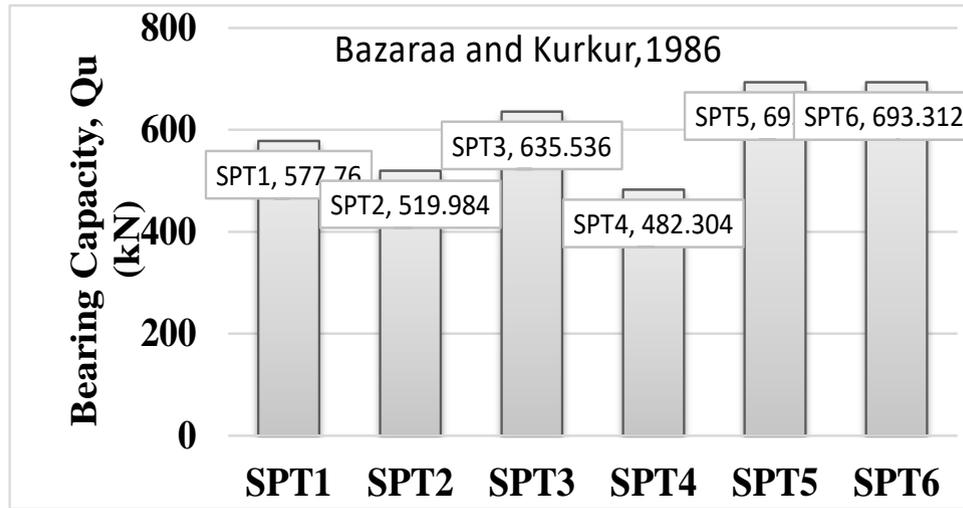
Fig. 7. Bearing capacity for proposed piles in all six profiles.
