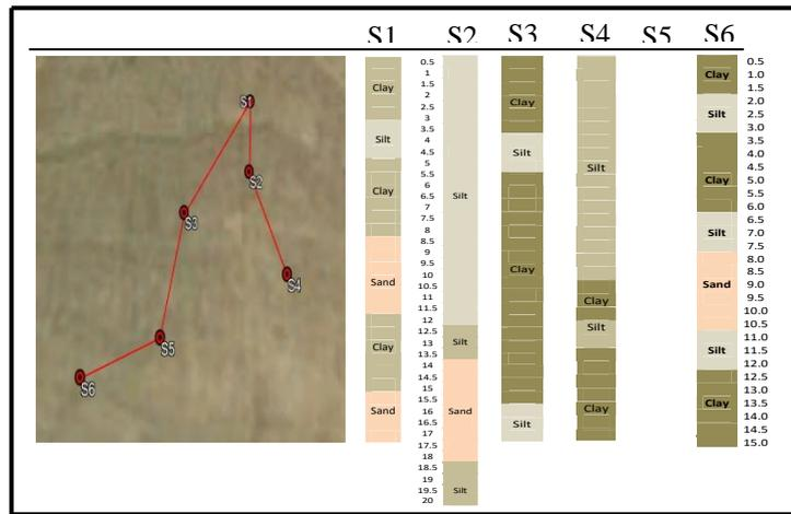
Fig. 2. The boreholes drilled in the site in addition to the location of these boreholes
