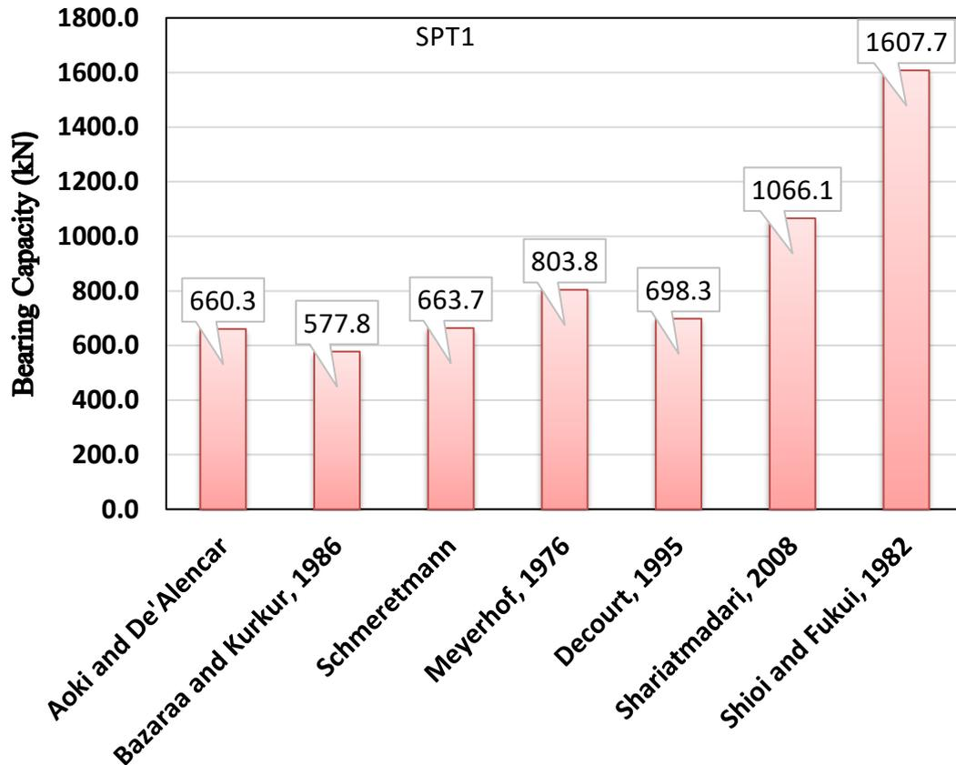
Fig. 5. Bearing capacity based on the results of SPT 1 using seven methods
