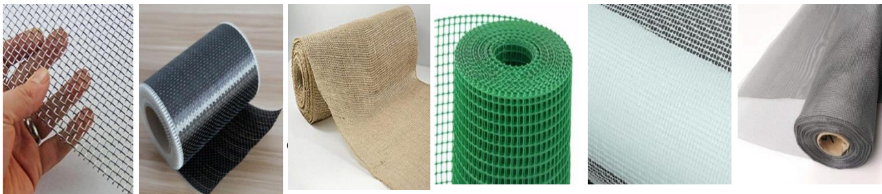
Fig. 1. Experimental setup and materials for fabric mesh confinement: (a) Steel wire mesh, (b) Carbon fiber sheet, (c) Jute fiber fabric, (d) 4×4 mm Polyethylene woven mesh, (e) 3×3 mm Polyethylene woven mesh, and (f) Window mesh fabric.
